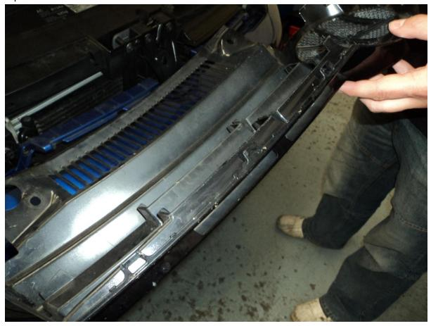
7. Undo the two T25 torx (one on each side of the bumper from where the grill was removed).
