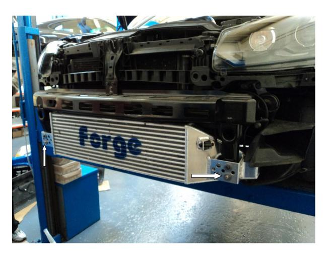
18. Now push the temperature sensor into the bracket on the intercooler.
