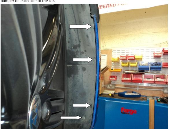
2. Undo and remove the T25 torx bolt found on the inner side at the top of the bumper. This holds the bumper to the wing on each side of the car.
