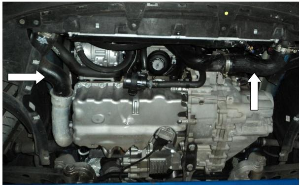
12. Remove the lower bar on the crash bar, by undoing the four T25 torx bolts. It should look like the picture below.
