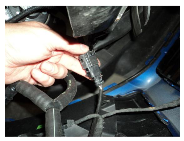
10. Next if you have headlight washers, these will need to be disconnected. To do this remove the "U" clip on the washer bottle pipe, situated on the driver side of the car and pull the connector from the pipe. You will need a bucket or bowl to catch the washer fluid.
