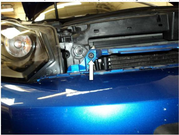
8. On both sides of the car pull down slightly and outwards on the corner of the bumper where it meets the wing. (READ THE NEXT 2 STEPS BEFORE DOING THIS AS YOU WILL SEE THERE ARE A FEW THINGS TO DO BEFORE THE BUMPER CAN BE REMOVED).
