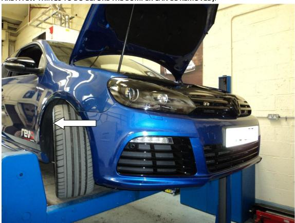
9. As you pull the bumper off you will have to remove some wiring. Firstly if you have parking sensors these will have to be unplugged (situated on the passenger side of the car), also on the driver side of the car you will need to remove the plug for the DRL's. Simply pull town on the tabs till you hear a click and then pull apart.
