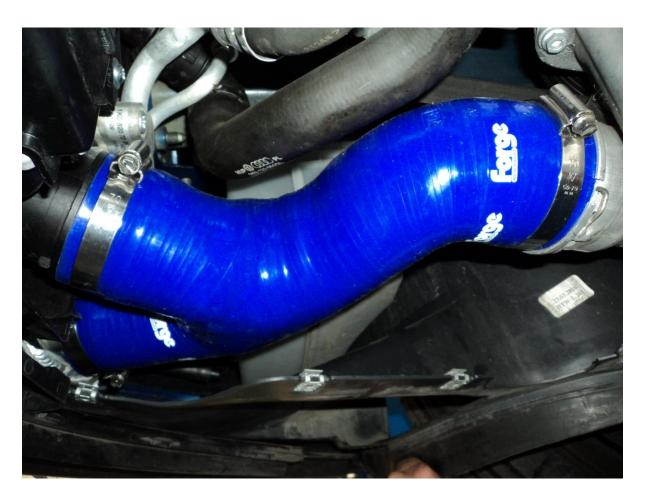
21. Under the car, remove the clip second from the front on both sides. This will stop you from using a screw in those holes of the undertray, as the silicon pipes are directly above this.
